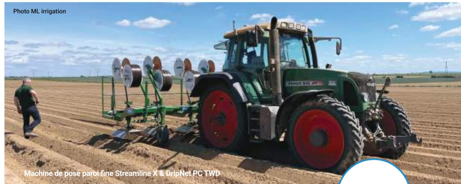
Machine de pose paroi fine Streamline X & DripNet PC TWD
